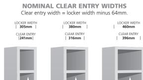
Allow up to 2.5mm per locker for horizontal creep
